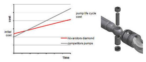
Maintenance: The Diamond series is designed to ensure easy maintenance and normally require the replacement of a minimum number of components. In particular the joint bushes allow the replace of the same without having to replace shafts and rotors. The costs of maintenance are really reduced. The cost of the pump, considered in his full life cycle, is highly competitive.
